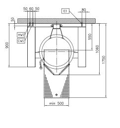
High Productivity Cooking Electric Tilting Boiling Pan, 100lt , Wall mounted with Stirrer The company reserves the right to make modifications to the products without prior notice. All information correct at time of printing.
